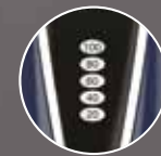
Digital battery indicator
