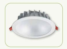
Ceiling cutout: Ø 145 mm, height 45 mm for 12 W. Ø 175 mm, height 55 mm for 15 W Ceiling cutout: Ø 205 mm, height 60 mm for 21 W. Ø 225 mm, height 65 mm for 25 W ORDERING: MODULE (MOD) + DRIVER (DRIVER TO BE ORDERED SEPARATELY)
