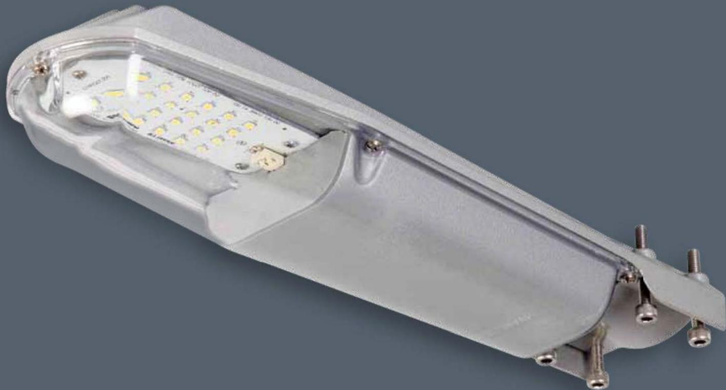
New generation energy saving and Environment-friendly long life LED street lights made up of pressure die-cast aluminium housing with high power LED as lighting source and lens embedded PC cover having TOP Opening seperate driver compartment with IP65 protection and impact resistance of IK07.
