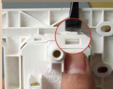
You can use screw driver to push it, and bring the lock on right position
